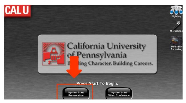
With the press of this single button, the projection screens will lower, the projectors will turn on, the lights will dim to the appropriate level, and the PC will be automatically displayed on both projection screens.
