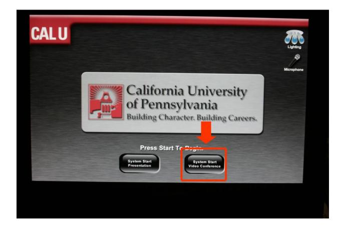
With the press of this single button, the projection screens will lower, the projectors will turn on, the lights will dim to the appropriate level, and the PC will be automatically displayed on both projection screens.
