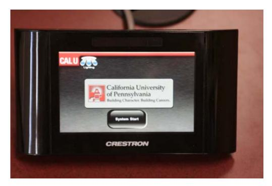
With the press of this single button, the projection screen will lower, the projector will turn on, and the PC will be automatically displayed on the projection screen.
